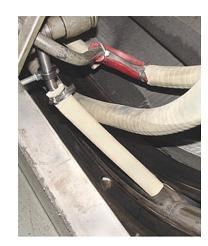
Please Note - Once mounting positions have been chosen, FIRMLY secure serrated flange nuts and hose clamp.
