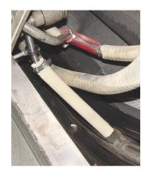
Please Note - Once mounting positions have been chosen, FIRMLY secure serrated flange nuts and hose clamp.
