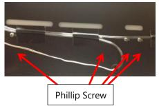
7. Before removing the tank assembly out of the lane machine, remove the tubing attached to the tank assembly along with the float switch assembly.
