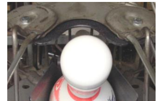
Top View Pin Head Guard at #5 position
