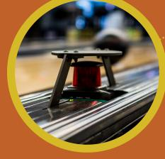
• Can be used with the FREE Specto Mobile apps and Coaches' App (PC) • Up to 40 data points to analyze • Lidar Sensor that captures about 60 readings per lane
