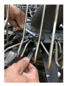
6. Install one 153-2052 bolt and one 153-2004 flat washer through the existing hole in the bottom turret plate as shown in the picture below. Place a 153-2004 lock washer and 153-2023 hex nut on the bolt. Thread the hex nut af few turns onto bolt. Do not tighten.
