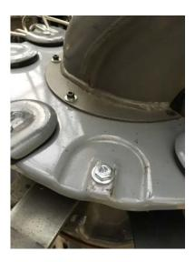
7. Install turret pocket and bracket assembly ensuring the flat washer is above the slot in the mounting bracket. Insert the bracket so the bolt is 2/3rds of the way into the bottom slot as shown in the picture below. Lightly tighten hardware with fingers. Install the additional hardware for the top of the bracket in the same fashion.
