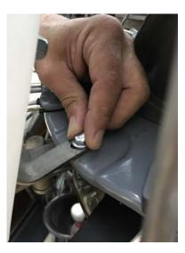
8. Rotate the spider assembly ensuring the spoons are in the locked position. Adjust the turret pocket left or right so it is perfectly centered over the spoon as shown in the picture below. Tighten hardware.
