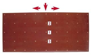
**2.** Drill three 3/32" pilot holes in the middle row hole positions, shown in above image, then secure with included screws.
