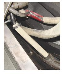
Avoid configurations that may allow neck of pin to be caught between Pin Deflector and lift rods. Example at left shows no space between lift rods gum rubber and Pin Deflector but some configurations can tolerate greater spacing from lift rods.
