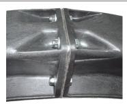
To install reinforcement ribs between pockets, place rib over pocket and insert spacers into both parallel (horizontal) mounting holes. Spread pocket 1/16" to align remaining hole and insert spacer.
