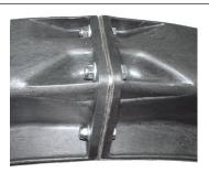
To install reinforcement ribs between pockets, place rib over pocket and insert spacers into both parallel (horizontal) mounting holes. Spread pocket 1/16" to align remaining hole and insert spacer.
