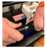
5. Remove the Oil Tip & Tube assembly from the machine by pulling it all the way out of the Flex cable carrier. Lay the assy onto a work bench.
