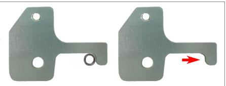
At 40-45 degrees, hook should fully rest on top of spacer as shown in image above left.
