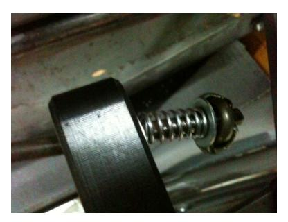
23) With the ball lift rod assembly resting in its normal position. Push the clamping collar onto the shaft until the first washer, coil spring, second washer and clamping collar are contacting each other and the first washer is contacting the nylon actuator arm. However  $\underline{DO\ NOT}$  push these parts together so much that the spring starts to compress. Back the clamping collar off the approx. 1/16 - 1/8" and tighten the bolt to clamp the collar to the rod.
