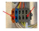
6. Remove the wires for the float switch plug to the wago block on the two spots (SHOWN LEFT). Do this by using a small screwdriver and pressing in on the top of block and pulling on the wire. The
