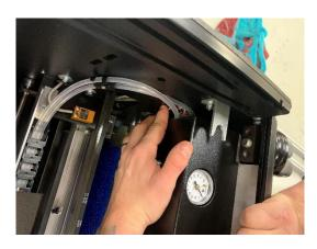
34. Add conditioner and run the pumps. Inspect for any leaks and that it is functioning properly.
