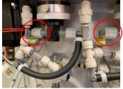
8. Remove the two fittings going from the bottom of the tanks to the left side of the oil pump assembly. Next, using pliers, unscrew the white knurled fastener counter-clockwise that is on the pump and pull the grey fitting out.
