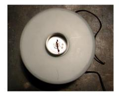
2. After marking everything inside the inlet, a reference mark will need to be put on the canister where it meets up with the plastic housing.
