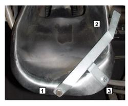
Using turnbar without extension mounting hole bolt [3] is not recommended.
