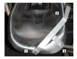
Using turnbar without extension mounting hole bolt [3] is not recommended.
