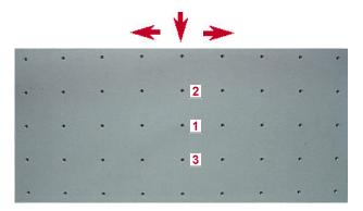
**2.** Drill three 3/32" pilot holes in the middle row hole positions, shown in above image, then secure with included screws.
