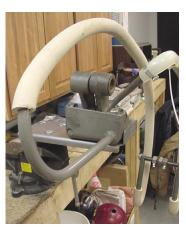
Remove clapper box height adjusting screw and firmly secure lift rods assembly under Lift Rods Bench Mount with provided (located above slotted hole) grade 8 bolt and thru-hard washer. Secure Lift Rods Bench Mount flanges, with mounted lift rods assembly, squarely into bench vise.
