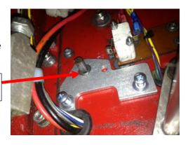
On ALL Walker models, it will be necessary to remove the support post as shown to the right. Failure to do so will cause potential damage to the transfer roller pulley and belt assembly.
