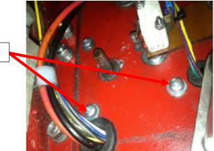
5. Locate the Buffer Mounting Bracket and mounting hardware from the kit. Install the bracket as shown to the right and fasten into place using the two screws, washer and lockwasher provided in the kit.
