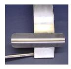
Snubber guide wire is important in keeping the 1, 7, or 10 pin from slipping out of the basket as the turret moves to the next position.
