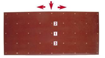
**2.** Drill three 3/32" pilot holes in the middle row hole positions, shown in above image, then secure with included screws.
