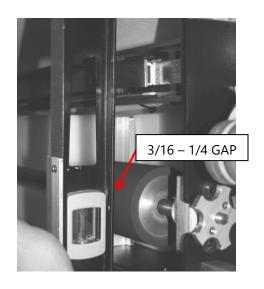
The **tilt** or **pitch** of the squeegee may also need adjustment to ensure that both blades are contacting the lane squarely. If a pitch adjustment is necessary, follow the steps below to make the adjustment. Make sure the squeegee motor does not bind up when making an adjustment. If the link is too short the motor cannot rotate 360°.
