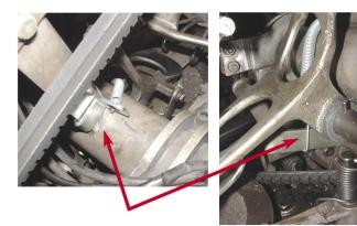
Blocking finger must move freely on shaft. Loosen with WD-40 or similar product and work pivot point until free, if needed.
