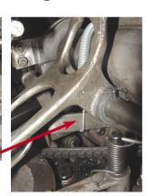
Blocking finger must move freely on shaft. Loosen with WD-40 or similar product and work pivot point until free, if needed.
