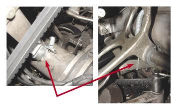
Blocking finger must move freely on shaft. Loosen with WD-40 or similar product and work pivot point until free, if needed.
