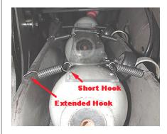
Each cross conveyer has its own lane conditioner carry down characteristics. The 6 supplied springs will be satisfactory for most cross conveyers. For extreme lane conditioner carry down add more springs (part #PPP-PPTS) in neighboring holes as needed.
