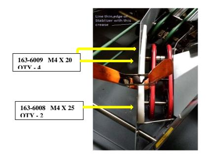
4. Drill mounting holes using the Crossover Wedge as a template. Install Crossover Wedge with hardware
