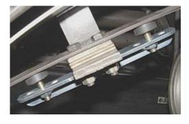
Shim Pin Wiper to obtain approximately ½ to ¾ clearance between wiper tip and turn pan. Fine tune by adjusting bumper positions.
