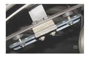
Shim Pin Wiper to obtain approximately ½ to 3/4 clearance between wiper tip and turn pan. Fine tune by adjusting bumper positions.
