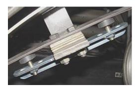
Shim Pin Wiper to obtain approximately ½ to ¾ clearance between wiper tip and turn pan. Fine tune by adjusting bumper positions.
